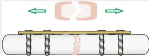
Fig/Animation 3.3.2-4 Perren's strain theory. A simple fracture (small gap) fixed with a bridging plate (relative stability) is exposed to movement (high strain). Fracture healing is delayed or will not occur at all. The plate will eventually fail.
